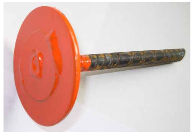
Fig. 1. Metal washers or steel discs can be welded to rebar stakes cut at an angle to create a permanent marker. It is highly recommended to paint the discs with implement paint (such as Kubota® orange pictured here) as it tends to endure the elements better than standard paint. Discs can be pounded into the ground and are level with the soil surface at the photo point.
