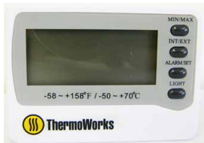
Fig. 1. Minimum/maximum thermometer (photo by Scott Jensen).
