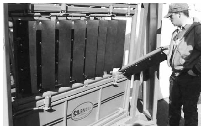
Fig. 9. Angled rubber louvers prevent cattle from seeing people standing next to the squeeze chute. Homemade louvers can be made from old round bailer belts. They are mounted on a 45° angle.
